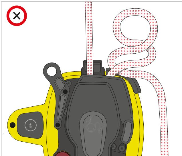
Stop immediately when a rope twist is observed, untwist and organise the rope before continuing.
