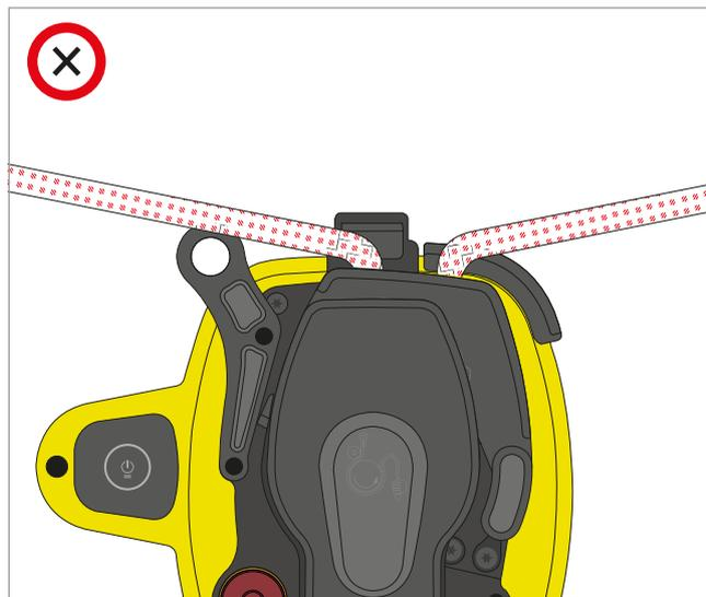
**The dead rope must never be loaded (in order to avoid side loading on the Rope Guide).** Do not build tramways using the primary rope as shown in the picture.
