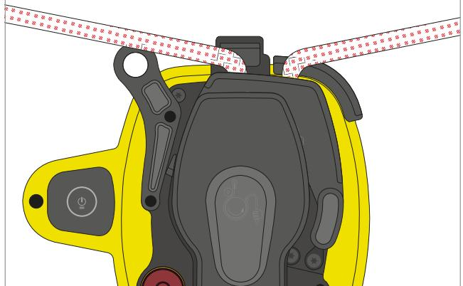
**The dead rope must never be loaded (in order to avoid side loading on the Rope Guide). Do not build tramways using the primary rope as shown in the picture.**
